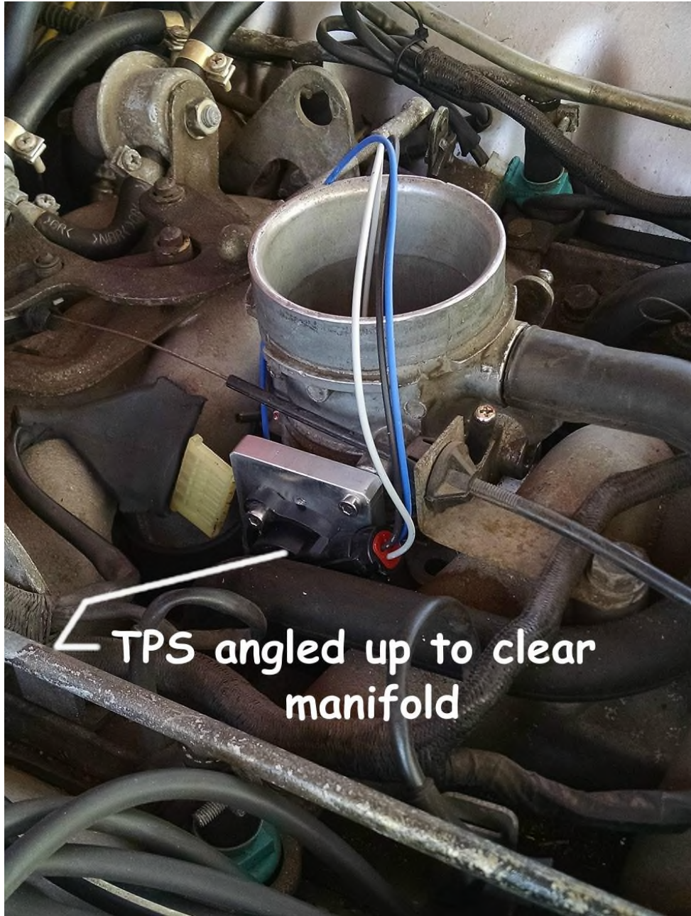
With the TPS position corrected, the throttle body is now reinstalled on the engine.
